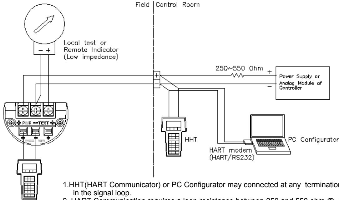
1. HHT(HART Communicator) or PC Configurator may connected at any termination point in the signal loop.
